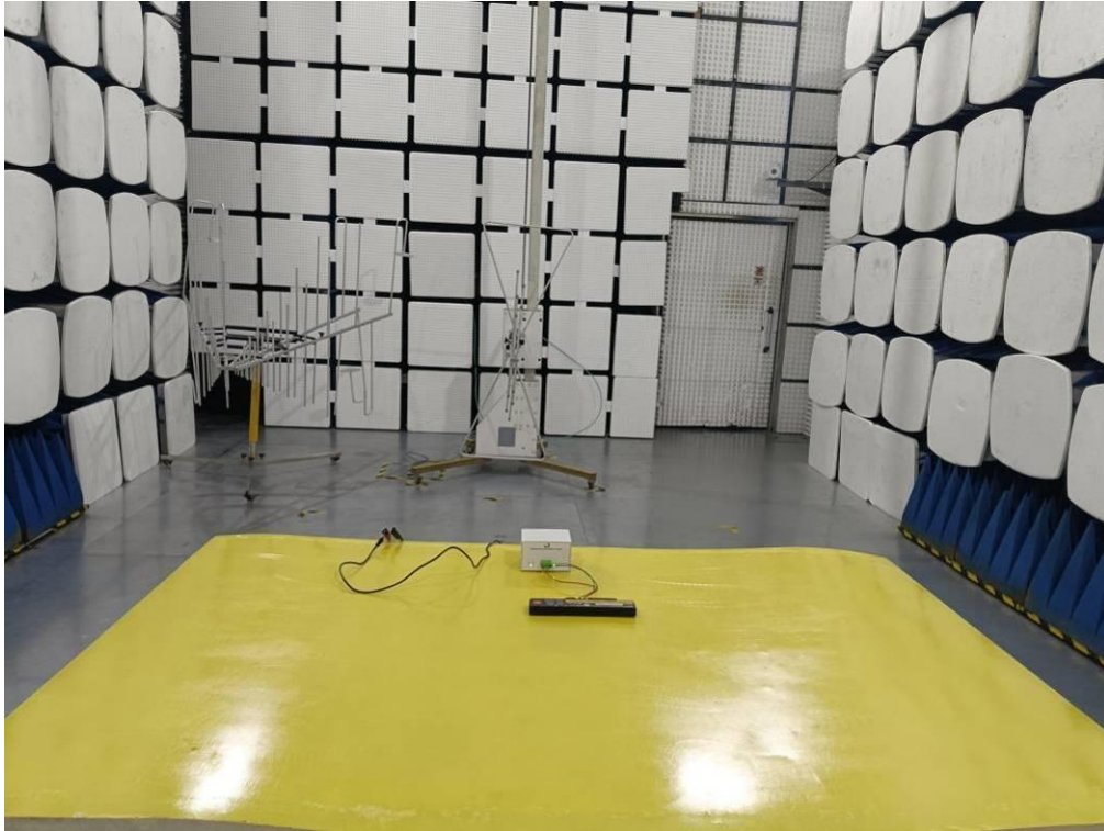
Photo of Radiated Measurement(30-1000MHz)
